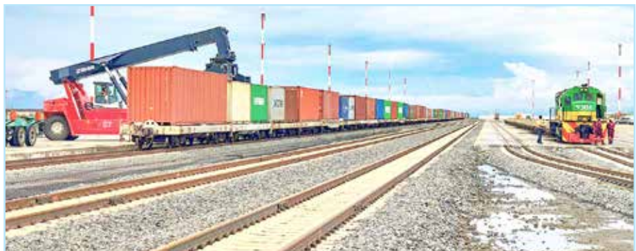
Transshipment of cargo from SGR to MGR at the Inland Container Depot (ICD) Naivasha.
